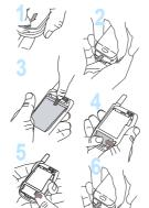
The SIM card is inserted under the phone's battery. Ensure that the phone is switched off and the charger disconnected.
